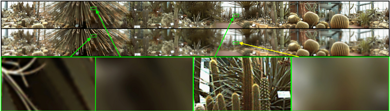
Figure 1: Images rendered from a 22 MPixels (spatial resolution: 17885x1275 pixels) panoramic light field at different focus settings (far: top, near: center), and close-ups in native resolution (bottom). We thank the Raytrix GmbH for capturing and providing the raw data.
